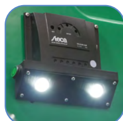
LED lamps lighting the tank interior.
